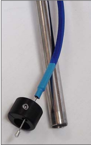
Figure 4.4-9 Remove the Cable Anchor at the end of the horizontal arm of the Right-Angle Tube and slide on the TUSB.
