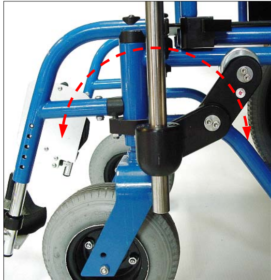
Figure 4.4-6 The LSAOP must be aligned vertically
