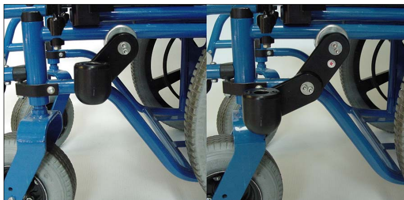
Figure 4.3-2 Each Offset Link provides three inches of offset adjustment.
