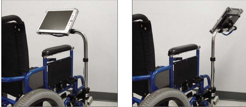
Figure 4.1-1 The DAESSY Locking Swing Away Mount on a power wheelchair
