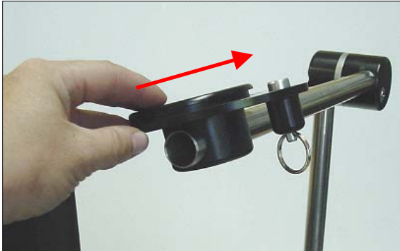
Figure 5.4-9. Slide the TUSB onto the Horizontal Tube and tighten the Pinch Clamp.
