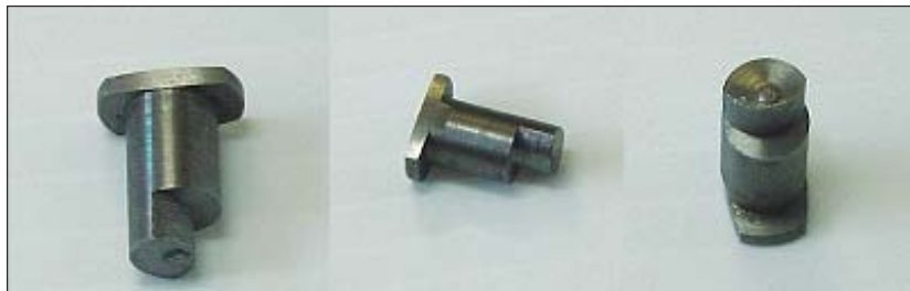
Figure 5.4-11 The slightly oval shape of the end of the Stop Pin shaft allows fine adjustment of the maximum movement of the Side Tube.
