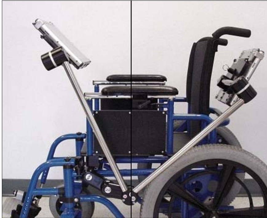
The DAESSY Rear Folding Mount DRFM6 in its In-Use and Folded positions.
