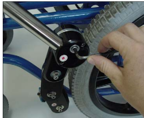
Figure 5.4-6 Tighten the Pinch Clamp bolt.
