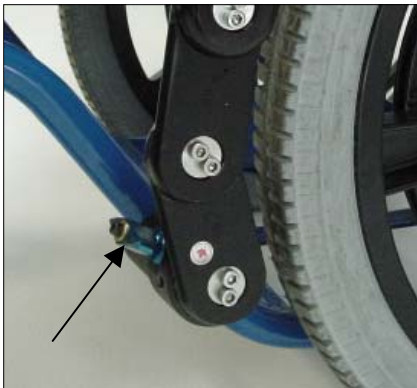
Figure 5.4-4 The RFCI-RFCR can be installed to allow easy removal of the mount.
