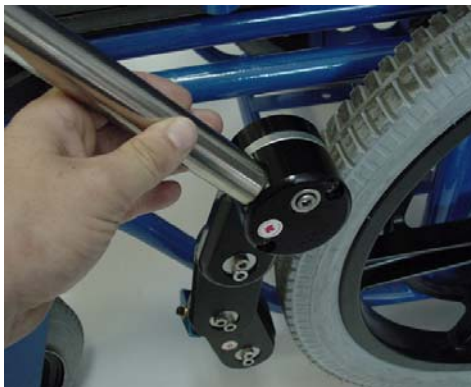
Figure 5.4-5 Align the Pinch Clamp and insert the Side Tube into the tube hole of the RTHTM.
