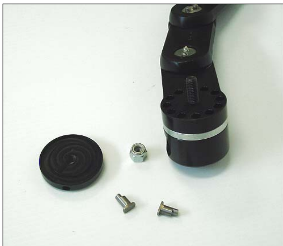
Figure 5.4-3 Unscrew the Locking Nut and Cover to remove the Stop Pins from the Rear Folding Adapter.
