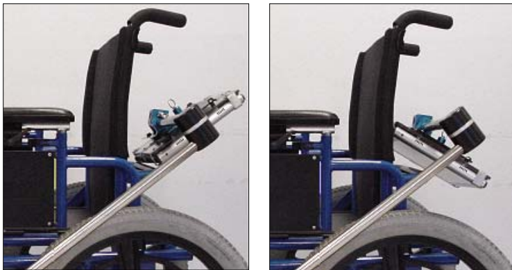
Figure 5.4-10 The Folding Quick Release Base (USBF) allows the device to be rotated around the Horizontal Tube and held at any of 5 angles by a spring-loaded lock pin.
