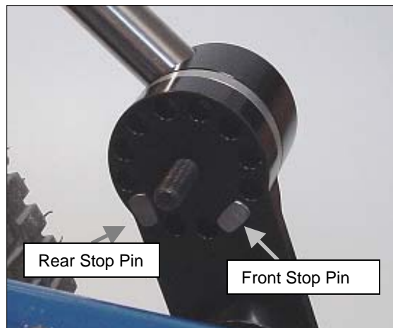
Figure 5.4-14 The Front and Rear Stop Pins must be align to seat in the groove in the Screw-on Cover
