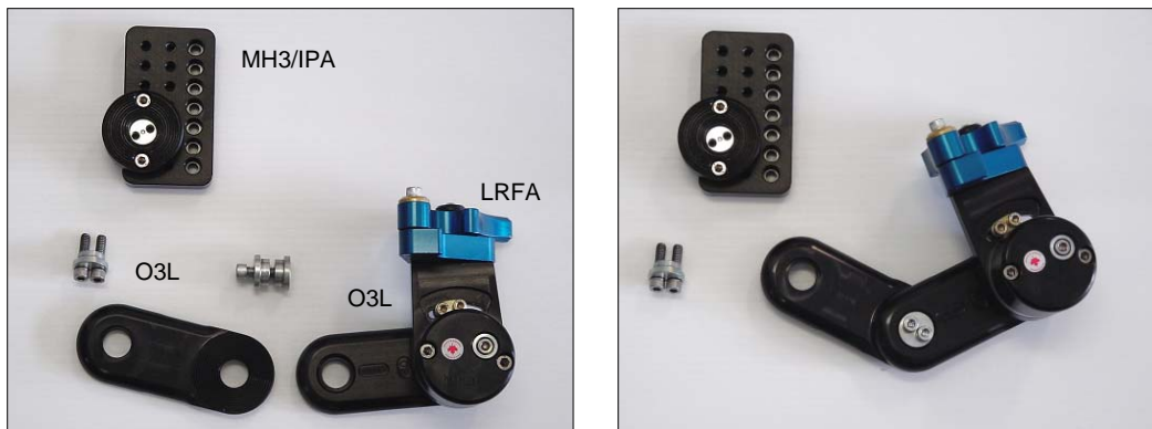
Figure 6.4-4 Unassembled and assembled Frame Clamp Assembly. The MH3/IPA bolt on adapter is first connected to the wheelchair frame, as the bolt heads may be obscured by the Offset Link of the Frame Clamp Assembly.
