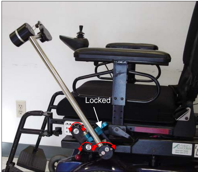
Figure 6.4-11 – With the Side Tube locked in place rotate the Locking Rear Folding Adapter at the Swivel Clamps connecting the Frame Clamp components to set the In-Use position.
