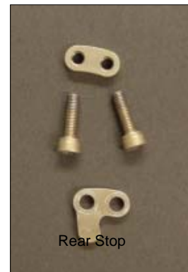
Figure 6.4-13 The Rear Stop can be removed and inverted to adjust the maximum rearward motion of the Side Tube.
