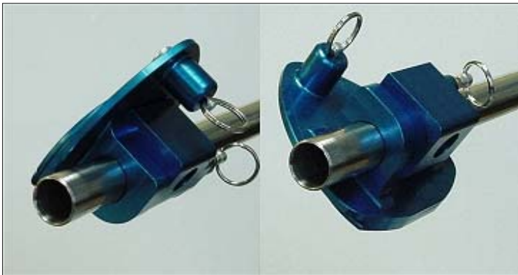
Figure 6.4-10 The Folding Quick Release Base allows the device to be rotated around the Horizontal Tube and held at any of 5 angles by a spring-loaded lock pin.
