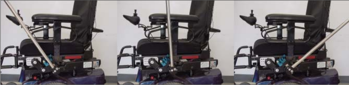
Figure 6.4-7 The Side Tube must not contact any part of the wheelchair as it rotates between the In-Use and Folded positions.
