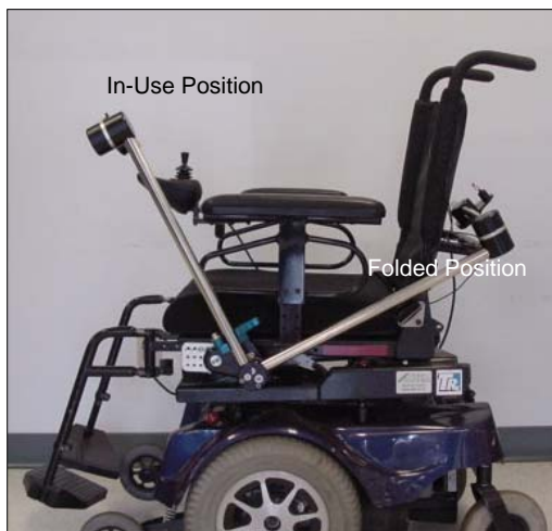
Figure 6.3-1 The In Use position is determined by the needs of the User. The folded position behind the backrest must be chosen such that the device does not interfere with other wheelchair fittings.
