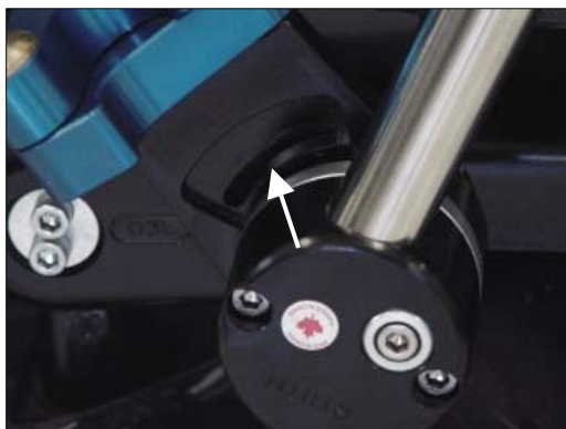
Figure 6.4-13 The Rear Stop can be removed and inverted to adjust the maximum rearward motion of the Side Tube.
