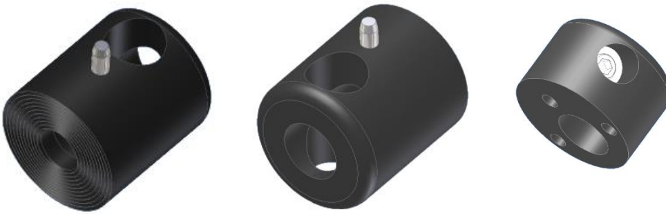
Figure 8.1.1 The standard Frame Clamp Outer Piece (UFCOP – two views) and Index Clamp (IC1) are used with the DAESSY Rigid Mount and DAESSY Folding Mount. Note the three index holes in the underside of the IC1 which receive the index pin of the UFCOP
