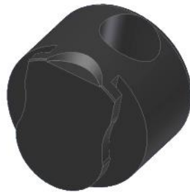
Figure 8.3.2. The Removable Outer Piece supports the Vertical Tube of the DRM1ROP and DFM2ROP
